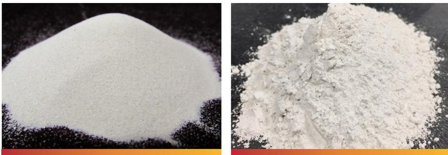
Zircon is almost exclusively used in the primary slurry and as a primary stucco. Because of its high density, zircon provides excellent flow characteristics in a primary slurry. The round grains do not cause defects such as rough casting surfaces.
