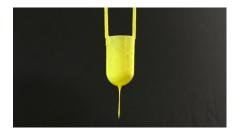
Through the hole: looking down into the cup, when daylight can be seen through the hole.
