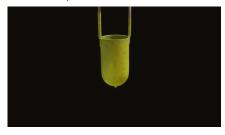
One inch below: watching from the side of the cup, when the slurry breaks one inch below the bottom of the cup.
