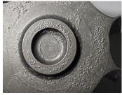
Air bubbles present as round or spherical metal defects or foam-like surface roughness.
